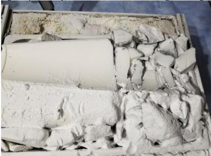
Figure 5. Salt lick test article post-test. Intact salt lick block (left) epoxyed salt lick pieces (right)
